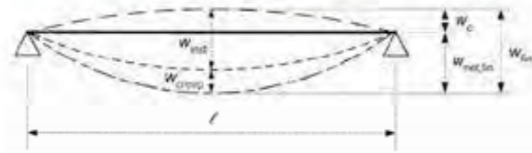
Figure 7.1 – Components of deflection
