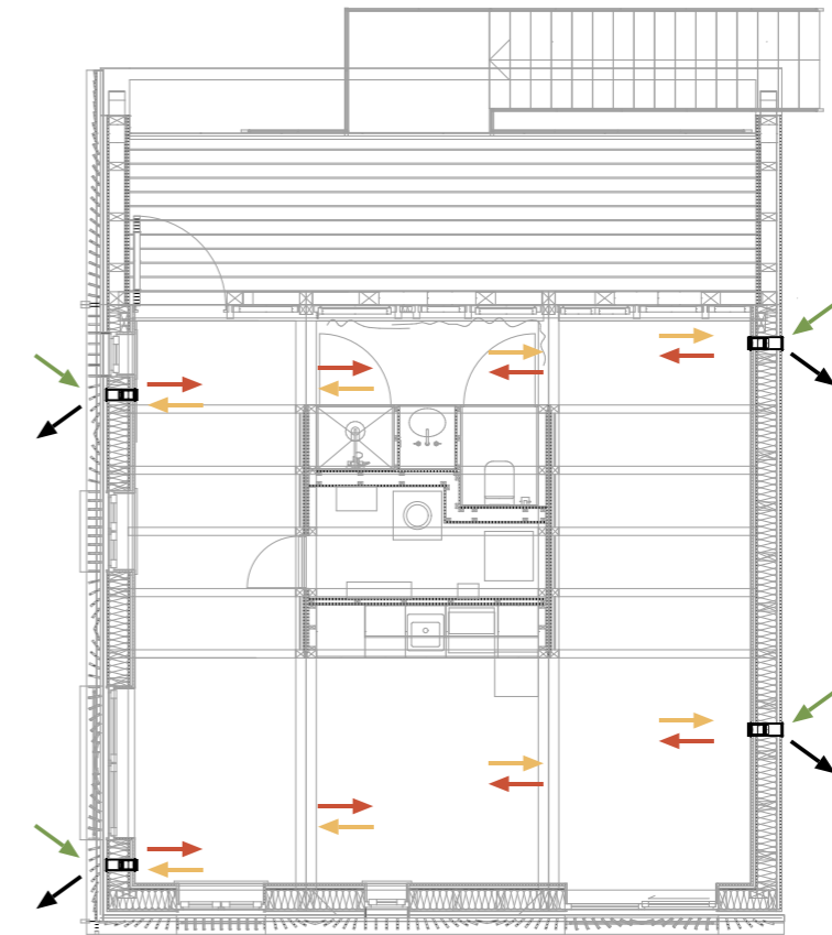
Fig. IV.2. 9. Decentralized ventilation systems in the HDU
