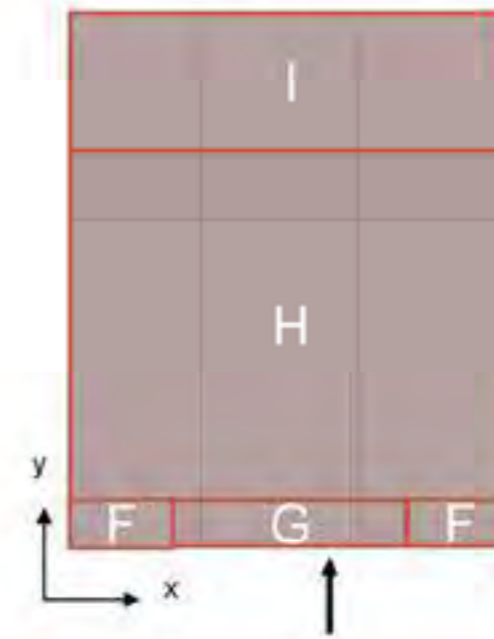
Figure 7.10 — Key to multispan roofs
