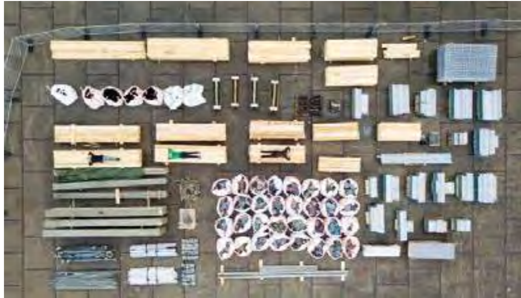
Fig. IV.5. 7. The People's Pavilion, Eindhoven Design week, 2019, bureau SLA + Overtreders W: all components can be dismantled
